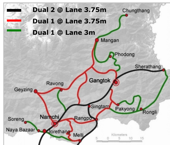
Figure 3.4.8 Proposed Hierarchy for Road Connections
