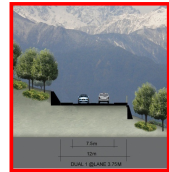
Figure 3.4.10 Proposed dual-1 road (3.75m) to be constructed
